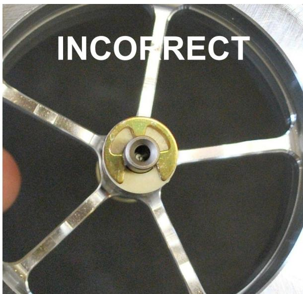
If you are having trouble installing the "C" clip correctly it may be bent. If it is bent the least little bit it will not seat itself into the groove properly and will come off. If you bend one we will gladly send you replacements. They are also available at most high end hardware stores.
